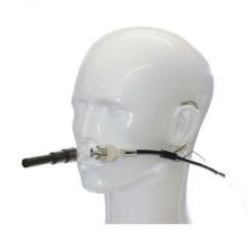
The SKC Face Level Sampling Headset is a personal air sampling media holder, featuring dual flexible sampling arms for parallel simultaneous samples and allows measurements inside personal protective equipment (PPE) such as masks and helmets, and is particularly suitable for sampling for hazardous metals in welding fume (such as manganese, nickel, chrome, etc) in welding applications.
